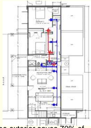
Blowing air from the inside towards the exterior saves 70% of the ducting – requiring significantly less energy to deliver the same volume of air.
